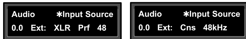
When the PCM 91 is receiving valid digital audio, selecting Input Source will display the input connector, audio format, and the rate of the incoming signal.
